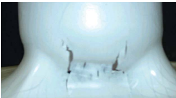
Figure 2 Fracture of the polymeric sheet during plug-assisted vacuum thermoforming. [Color figure can be viewed in the online issue, which is available at www.interscience.wiley.com .]
